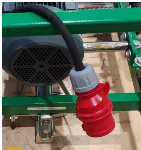
connect wheel spinner with electrical panel box using included cables
